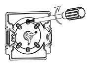
7. Fix the fixture by 4 screws
